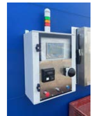
Simple and intuitive operator panel. Status of the system and instructions for the operator constantly displayed on the screen
