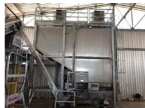
ICESILO version with stainless steel insulation
