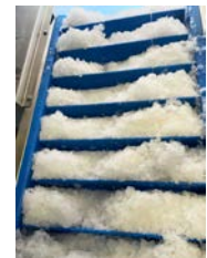
Ice transport on conveyor belt
