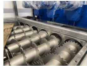
Variable pitch helical screw conveyors to avoid the compression of the ice
