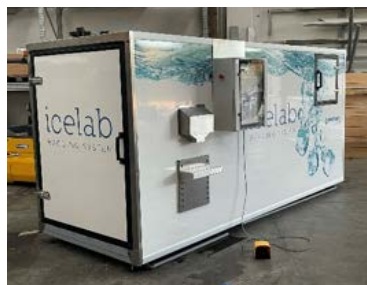
Interlocked access door for cleaning and maintenance operations
