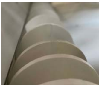
Extraction with worm screw with variable pitch made of food plastic material
